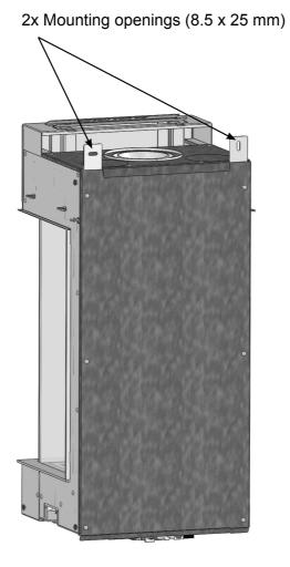
Figure 21: Mounting openings (2x) Rear Wall-mounted appliance
