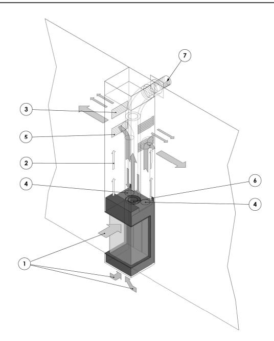
Figure 18: <u>WALL-MOUNTED APPLIANCE</u>: <u>Appliance with ventilated cove</u> Horizontal outlet of the flue gas exhaust /combustion air supply via the wall. Fitted with the options / accessories:
