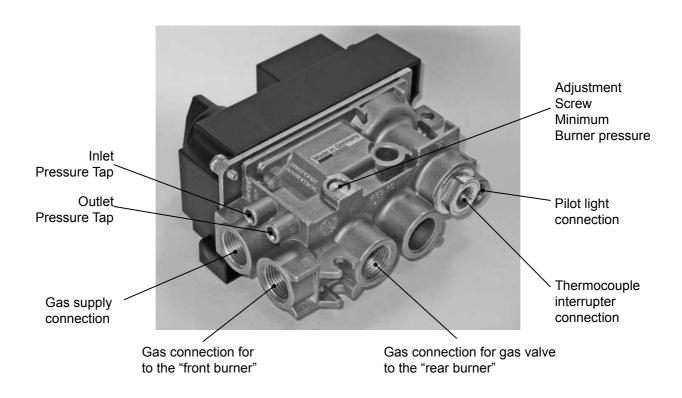
Figure 25: Gas regulator block - Rear
