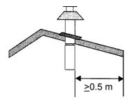
Figure 1: Roof-mounted outlet
