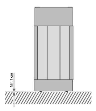
Figure 15: A clearence of at least 1 cm must be maintained between the bottom of the appliance and the floor.
