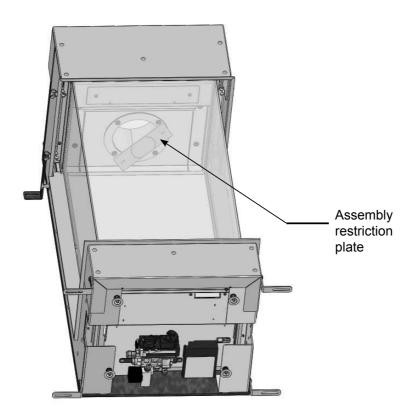
Figure 32: Positioning restriction plate
