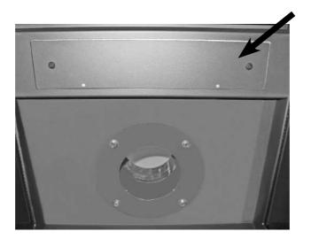
Overpressure hatch is in the correct position.
