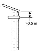
Figure 2: Wall-mounted outlet
