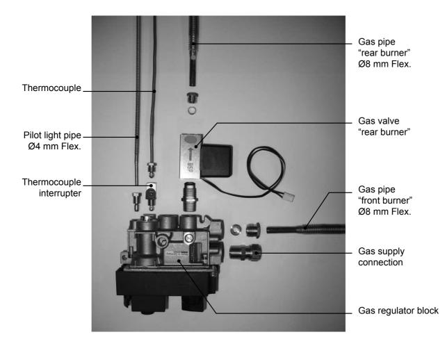
Figure 23: Gas regulator block and gas valve: Gas and thermocouple connections
