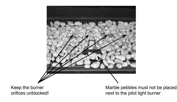
Keep the burner orifices unblocked!
